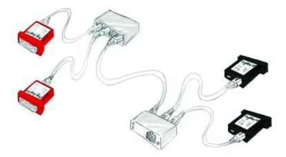
This mode is used to bridge large distances, isolate devices electrically or use existing networking infrastructures. All streams originating from StageFeed ISP converters are combined with an Ethernet switch and transmitted across copper or fiber cables. Then split by a second Ethernet switch and fed into the StageMate ISP converters. The mode can be used to replace ISP-DB25 splitter cables by configuring StageFeed to establish multiple bridges.
