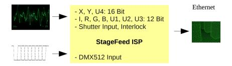
For its network output, the converter implements a preliminary version of IDN, the ILDA Digital Network protocol currently under development. The converter captures its analog inputs simultaneously and transmits a stream of samples, packed into IP-packets, to configured and/or registered hosts.
